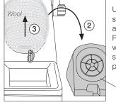
Unlock the splashguard (1) and take it off (2). Replace the worn wool (3), put the splashguard in place and close it.
