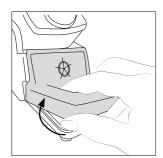
Lift the wiper at its front edge.
