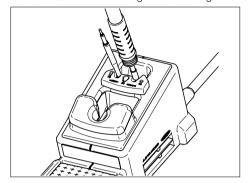
1 - Place the handpiece and remove the cartridge.
