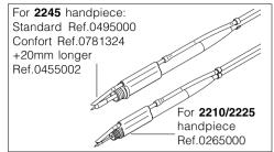
Specially designed for the Advanced Series 2210/2225 and 2245 handpieces. Easily clips onto the handpiece and can be quickly removed for easy maintenance.
