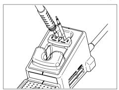
2 - Place the handpiece on top of the new cartridge, press it slightly down and remove the handpiece.
