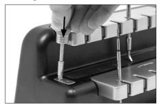
Use the hole that best fits to the cartrige tip dimension and push the handel down as far as the mark\*.
