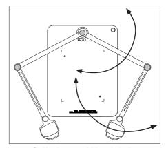
Position the arm and tighten the knobs.
