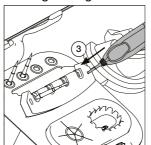
Gently press the tip against the holes on the sides of the cartridge exchanger (3) to ensure that the cartridge is appropriately inserted.
