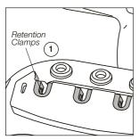
The cartridge exchanger allows to insert / change cartridges safely without switching the tool off. Cartridges are held in place thanks to the retention clamps (1).
