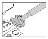
If Sleep Mode is activated (see section "Settings"), upon placing the tool in its holder, besides charging it enters Sleep Mode. The tip temperature drops down and remains at Sleep temperature.
