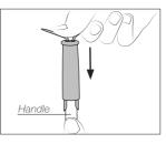
Push the grip with the fitters onto the handle.
