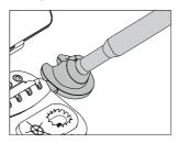
While the tool remains in the tool holder, it charges and the tip gradually cools down to room temperature.
