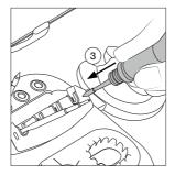
Make sure that the cartridge is appropriately inserted\* into the tool by gently pressing the tip agains the holes on the sides of the cartridge exchanger.
