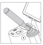
Place the tool in the charging holder (4) to charge it. A beep will sound to confirm that the tool is properly placed and charging. The sound can be turned up, down or off using the left button on the display.
