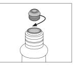
OB5000 has a thread for attaching the plug to the handle.
