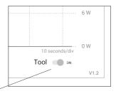
**Note:** The tool can also be switched off/on manually. Tap the *Tool* power switch on the display (bottom right) to switch it off/ on (if the tool is turned off, it will remain connected up to 5 minutes to the station but will not heat up the cartridge).
