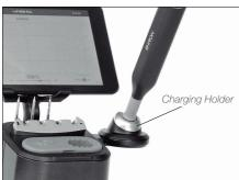
To reactivate and turn on the handle, the cap must be removed and the handle inserted in the charging holder so that the station recognizes the handle.
