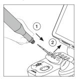
Place the tool over a cartridge and press the tool down to insert the cartridge (1). To release the tool with the cartridge from the extractor, lift the tool upward (2).
