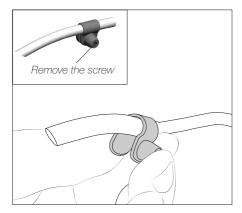
1. Unscrew the suction nozzle's clamp and take out the screw. Make sure that the nut and the suction nozzle stay in place.
