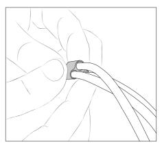
**4.** Use the tube clamps to hold all the tubes and cables so that they are more manageable and tidy.
