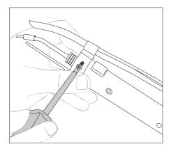
**3.** Once the suction nozzle is in the desired position and angle, use the screw to fix it in place.
