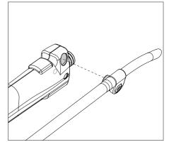
Assemble the suction nozzle and the clamp to the tool by matching the protrusion of the clamp with one of the side hollows of the tool (2).
