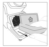
Remove the wiper by pulling it out.
