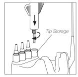
To remove the tip from the spanner, simply place the tip in one of the holes of the tip storage, screw it in lightly (only aprox. 1 turn) and pull the spanner out.
