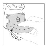
Lift the wiper at its front edge.
