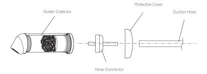
Reassemble the whole solder-collector group onto the desoldering tool.
