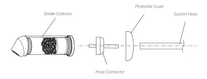
Reassemble the whole solder-collector group onto the desoldering tool.
