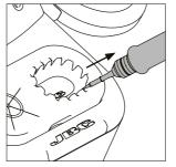
Use the slots to remove remaining particles.
