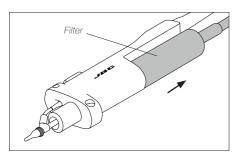
**3.** Use the cleaning brush (ref. 0008297) to clean the solder collector inside or replace it with a new one.
