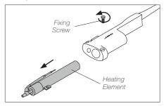
3. Insert the new heating element into the tool.
