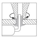
When the solder joint liquifies gently describe circles around the pin. Using the pin as the center of your movement.
