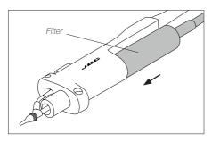
2. Take out the solder collector with the metal solder retention.
