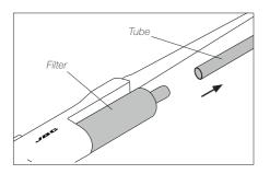
2. Remove the filter form the tool.
