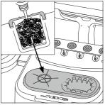
**CL0300** Brass Wool is a very effective cleaning method. It leaves a small layer of solder on the tip, preventing oxidation between cleaning and rewetting.
