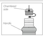
Position the chamfered side upwards and screw the new sealing plug into the handle bushing until it stops.
