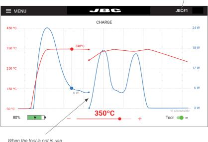
When the tool is not in use the graph stops recording
