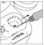
Use the slots to remove remaining particles.
