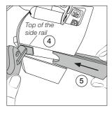
To install a new charging holder, place it at the top of the side rail (4) and slide back the slide band (5) until the holder is secured in place. Finally tighten the screws at the base.
