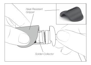
It is recommended to use the heat-resistant gripper to handle the solder-collector if it is still hot. The gripper's shape adapts perfectly to that of the collector.
