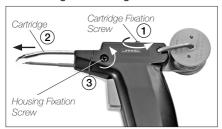
Loosen the cartridge fixation screw (1) and take out the cartridge (2). Loosen the housing fixation screw just slightly (3).
