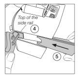
To install a new charging holder, place it at the top of the side rail (4) and slide back the side band (5) until the holder is secured in place. Finally tighten the screws at the base.
