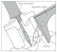
The system detects when the tool is returned to the stand and the fume will be automatically absorbed via the aspiration intake (4).
