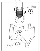
First remove the hose by twisting it (1). Shake the hose to get rid of the dirt inside.
